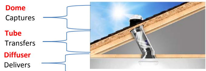
Fig. 1. A section through the roof of a building with a Solatube daylighting device
